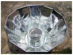
sections are held together with flexible tape hinges. The bottom is a round piece of polycarbonate covered with aluminum foil.
