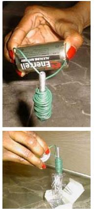
To use the electromagnet we held the ends of the coil of wire against the battery and lifted some paper clips. This electromagnet lifted 21 paper clips. These were the same paperclips that we used for the Clay Boat challenge.
