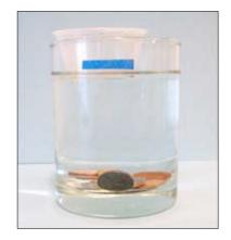
Before we look at our barge, imagine a block of wood floating in water. Since wood is less dense than water, it floats, partly above the waterline and partly below. The part below has displaced an amount of water that weighs the same as the whole block of wood.
