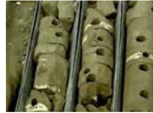
Core samples of reservoir rock taken during process of drilling an oil well
