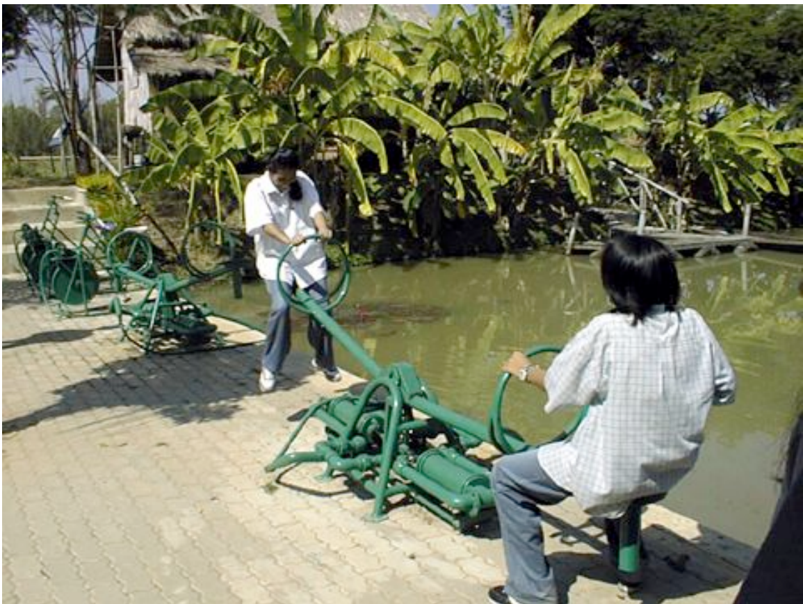
Energy created from this see-saw drives a water pump in a village in Thailand.
